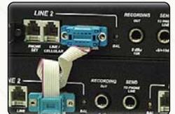
A flat cable **LINK** at the rear panel allows future enhancements.
