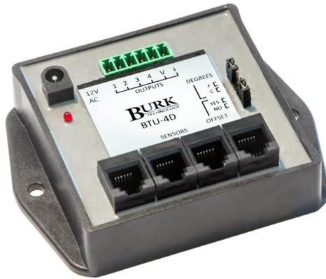
The BTU-4D Burk Digital Temperature Unit connects up to four digital temperature sensors to an ARC Solo remote control or to a Plus-X input device in an ARC Plus system. Sensor cables up to 1000 feet long are supported without measurement degradation. The unit also provides a low voltage output sample that tracks linearly with the AC line voltage.
